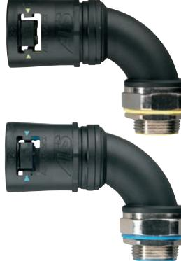
**90° Elbow fitting - Swivel external male thread / Materials: Polyamide (nylon) 66, nickel plated brass thread/TPE / Colour: Black (BL) / Yellow (Y), Blue (B) Elastomer**
