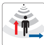
Radial and tangential Ideal for movements at right angles to and directly towards the sensor
