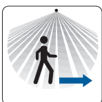
Tangential Ideal for movements at right angles to the sensor
